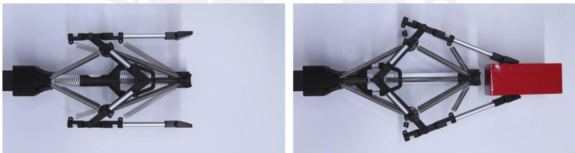
Figure 1-5 Gripper application of a tensegrity structure (Images from Sumi et al., 2017)
