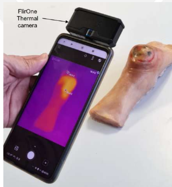
Figure 3.6: Illustration of the FlirOne Pro thermal camera attached to an smartphone for obtaining thermal images of a wound phantom.
