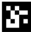
Figure 6.8: A sample of an ArUco marker. The ArUco marker is easy to detect by well known algorithms implemented in opencv.
