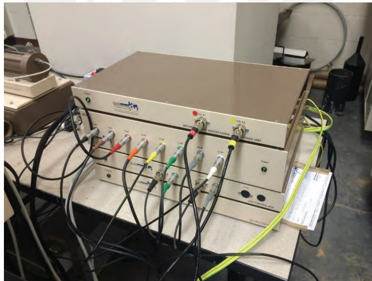
Figure 3-3: Data Acquisition boxes: From top to bottom: Bender Element controller, DCS and LVDT signal conditioner
