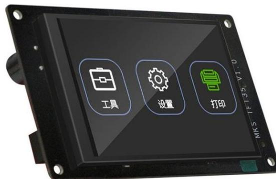
Figura B13-2: Pantalla táctil TFT. (Lankeda, s.f).
