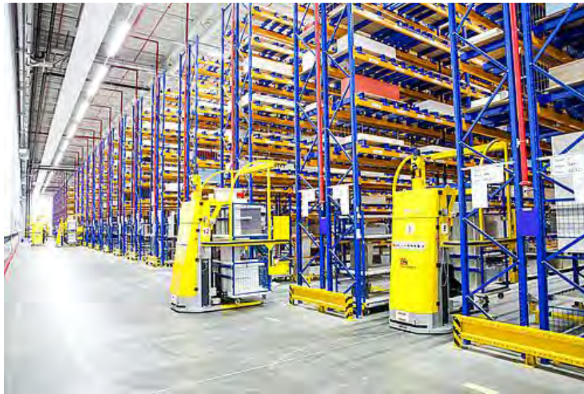
Figura 1.16. Grenzebach Automated Guided Vehicles (AGV).
