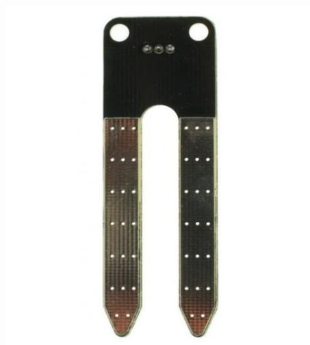
Figura 4: electrodo sensor FDR [11]
