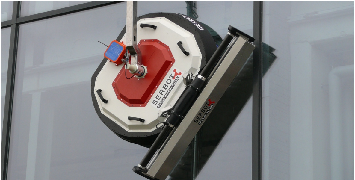
Figura 2. GEKKO Facade Robot
