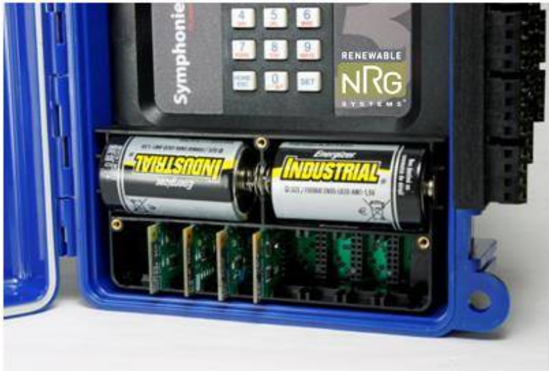
SCM cards installed under battery cover
