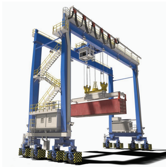
(c) Gantry crane [9]
