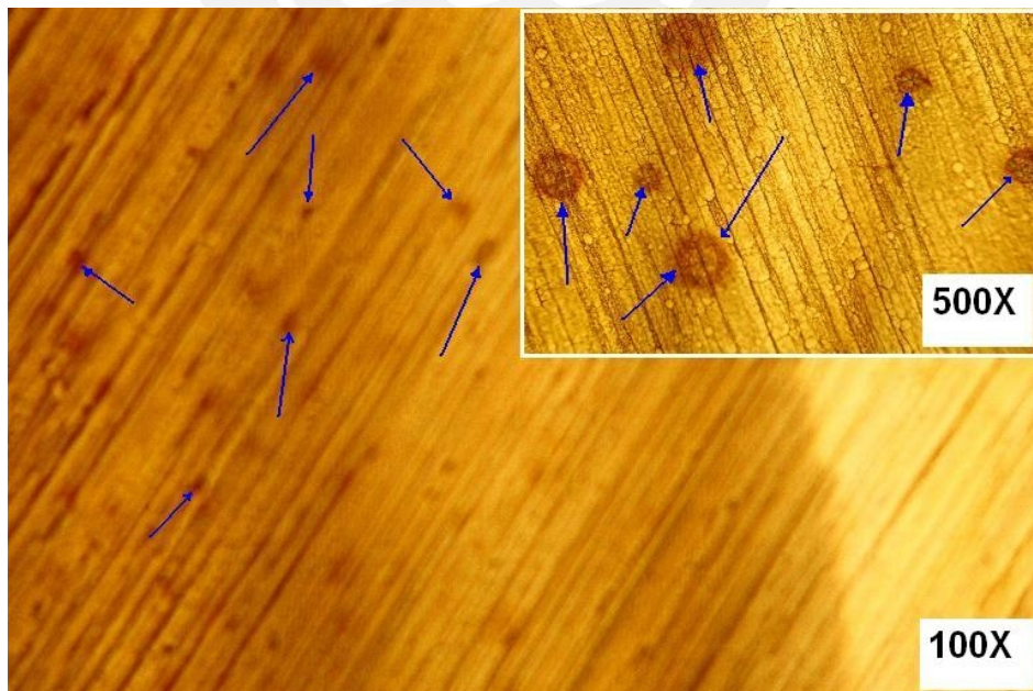
Deposit S1 after potentiodynamic anodic polarization
