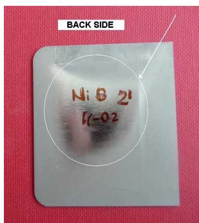
Figure 32. Back side of a substrate after Ni-P-SiC electroless deposition showing a zone with poor SiC incorporation
