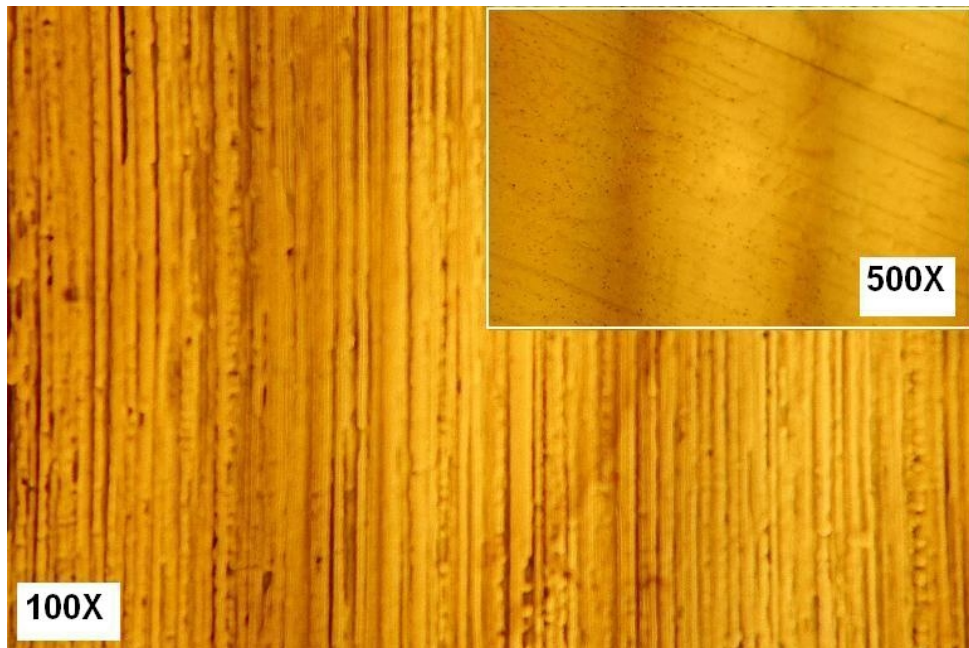
Deposit S1 after potentiodynamic anodic polarization
