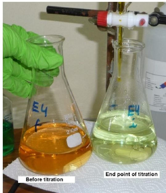
Figure 17. Hypophosphite determination by titration with Cerium (IV)
