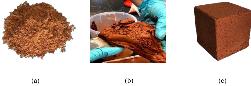
Figure 3.4. Production process of geopolymers: (a) FCBP; (b) FCBP geopolymer paste; (c) FCBP-based geopolymer cubic sample.
