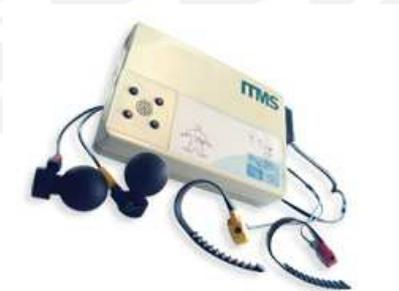
**FIGURA 2-1: ELECTROCARDÍOGRAFO PORTÁTIL**
