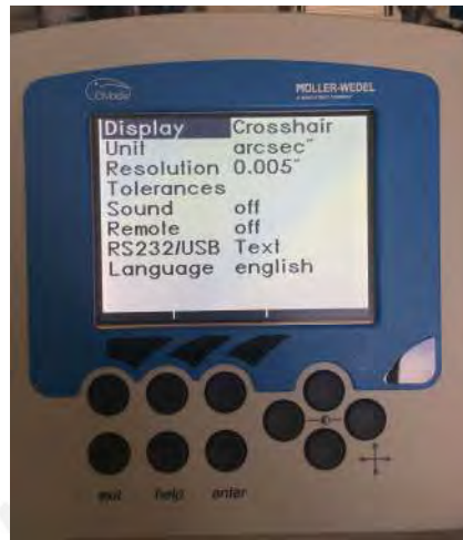
Figure 3.18.: Control unit of Elcomat 3000 - configuration display
