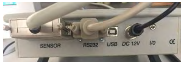
Figure 3.17.: Control Unit of Elcomat 3000 - Connections
