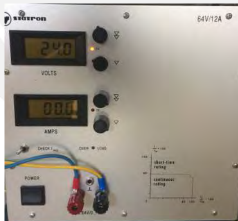
Figure 3.14.: Power supply Statron 64V/12A
