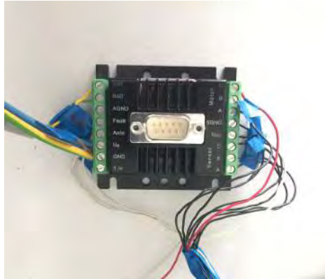
Figure 3.15.: Faulhaber controller - connections
