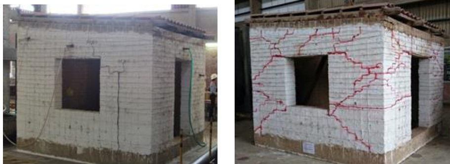
Figure 7. Adobe model before and after the intense shaking table test
