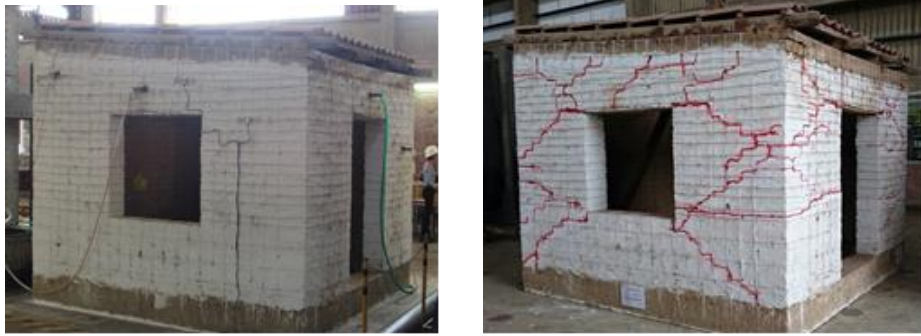
Figure 8. Adobe model before and after the intense shaking table test
