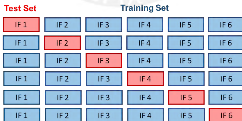
Figure 3.47: Inner-fold training and test set combinations. In the inner-fold training, each inner-fold is used once as test set while the other five inner-folds build together the training set.
